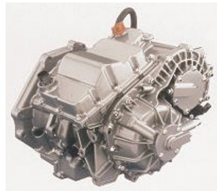
Figure (4) – GM’s New CVT design From [6]
